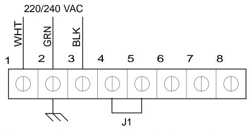
Fig. D2 - TYPICAL SIGNAL DEVICE WIRING
